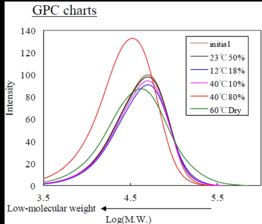
Have tried artificial aging at various combinations of temperature and humidity:
