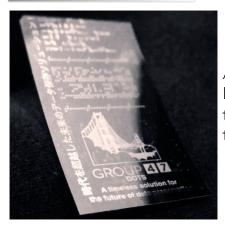
A photo of a test write to DOTS media, illustrating the ability to write binary, text, and images.
