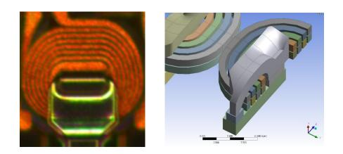
IBM developed a **new high moment (HM) layered pole write head** that produces much larger magnetic fields enabling the use of smaller magnetic particles
