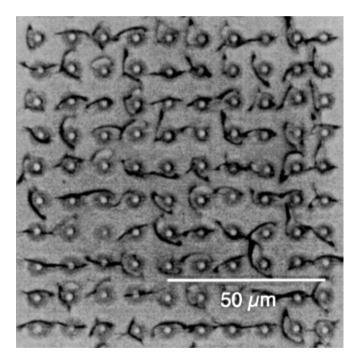
Femtosecond (100 x 10<sup>-15</sup> s) laser induced *small* voids in quartz glass
