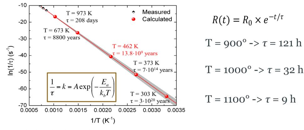
Using the Arrhenius law, the lifetime can be extrapolated to the room temperature
