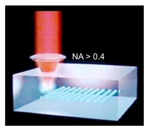
Intensity ~  $5x10^{13}$  W/cm<sup>2</sup> Electron temperature ~  $10^{5}$  K /10 eV Pressure ~  $10^{6}$  bar
