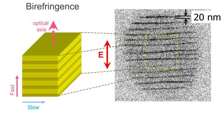
Femtosecond laser nanostructured glass:  $n_e - n_o = -5 \times 10^{-3}$
