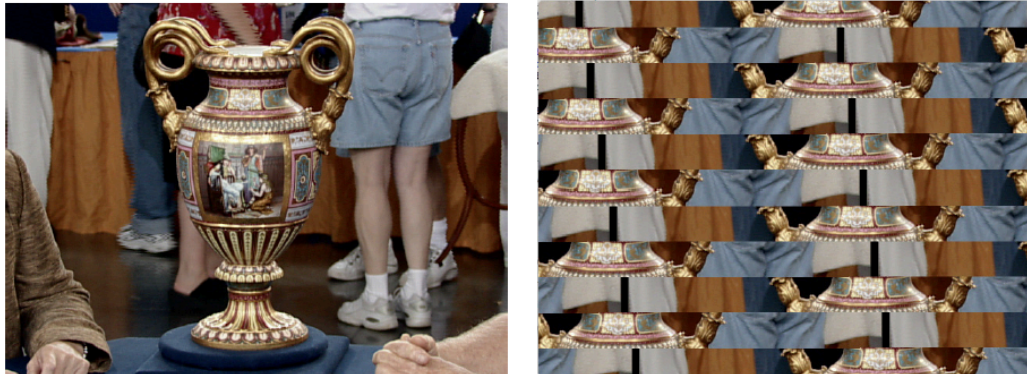
QC Failure: File reads as normal when tested, but content is replaced with repeated glitching image or green screen a portion of the way through the video
