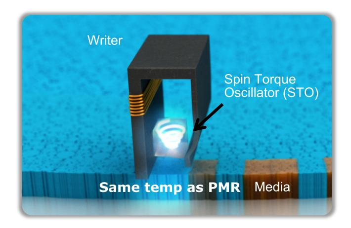
Microwave fields emitted by a Spin Torque Oscillator (STO) located near the write pole allows writing of perpendicular media at lower magnetic fields
